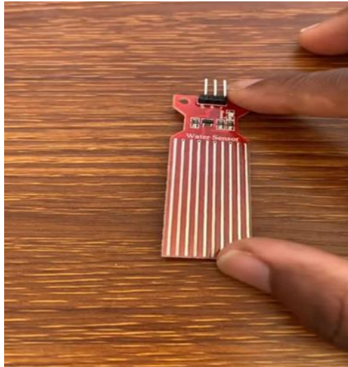
Gambar 6. Water Level Sensor
